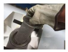
While the cylindrical filter is removed, place the wash gun in the drain, set the wash gun to "JET", rotary dial selection to RINSE TUB and flush the drain. Run the water gun for 20 seconds, if there are issues with the water draining away you may need to contact your plumber. Replace the cylindrical filter, and put the stainless-steel filter back into position.
