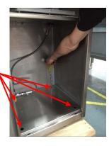
There are 2 different types of adjustable feet, four\* exposed that are adjusted by hand turning the actual feet and four\* inside the cabinet floor that have rubber grommet covers, you will need to remove the rubber grommets and adjust these with a large flat head screw driver.
