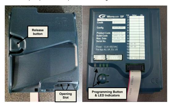
The photo above right shows the coin acceptors On-Board Programming (OBP) facility, refer to the following sections in its use.
