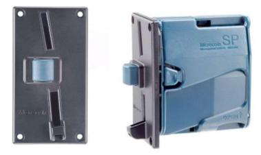
The below photos show both sides of the coin acceptor after it has been removed from the cash box.
