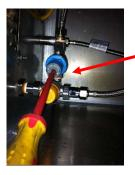
The picture left shows regulator being adjusted in a Compact with no hot water system on board.
