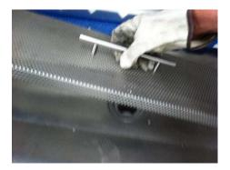
Warning the stainless-steel filter can have sharp edges, "rigger" gloves need to be worn to protect against injury. If required, you can wear rubber gloves underneath the "rigger" gloves.
