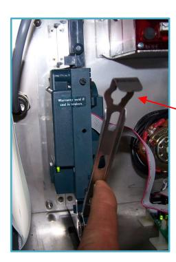
With bracket down, the coin acceptor will slide from its mount. Disconnect the small ribbon cable form the interface board as shown on right.
