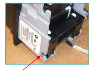
To remove the lower sensor block, raise the locator pin shown above and slide the sensor block out
