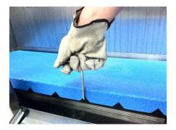
To lift the dog wash floor, open the dog entry door, using the tool as shown above, slide the hooked end under the front edge of the floor and slide sideways until the hooked end locates into one of the notches in the front edge, then lift.
