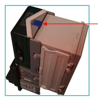
To remove the stacker from the note acceptor, press the blue catch forward and slide the rear compartment up.
