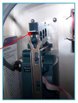
Once the bracket slides up slightly, pull it backwards towards you. This bracket is hinged on the bottom and will simply pivot. See photo on left.
