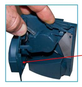
Open the side completely as shown on the left. This will allow ease of cleaning.
