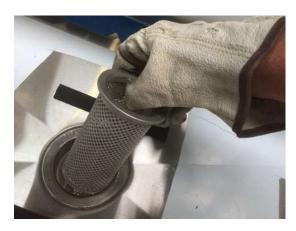
While the filter is removed, place the wash gun in the drain, set the wash gun to "JET", rotary dial selection to RINSE and flush the drain. Run the water gun for 20 seconds, if there are issues with the water draining away you may need to contact your plumber. Replace the cylindrical filter, and put the stainless-steel filter back into position.
