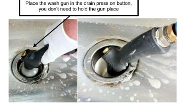
Turn the wash gun back on, select the disinfect option on the rotary dial and wash the under-floor area, return tilt floor to the down position. While still on disinfect, wash down the tub area of the dog wash. Turn gun off, remove wash down key and select the stop option on the rotary dial.
