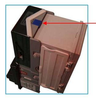
To remove the stacker from the note acceptor, press the blue catch forward and slide the rear compartment up.
