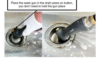
Turn the wash gun back on, select the disinfect option on the rotary dial and
