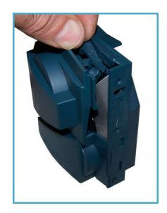
Open the side completely as shown on the left. This will allow ease of cleaning.
