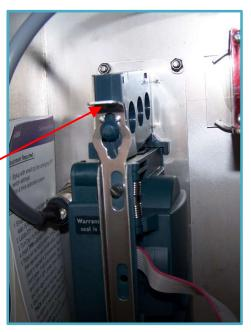
Once the bracket slides up slightly, pull it backwards towards you. This bracket is hinged on the bottom and will simply pivot. See photo on left.
