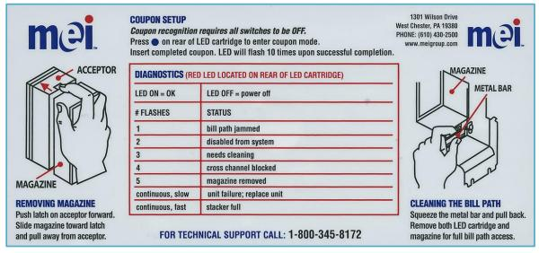
The magazine that holds the Notes must be clipped into its normal position to ensure you get an accurate fault code.
