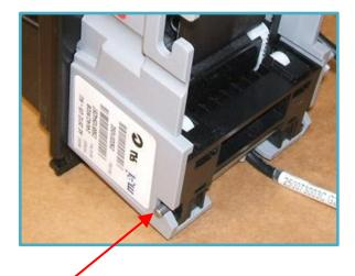
To remove the lower sensor block, raise the locator pin shown above and slide the sensor block out
