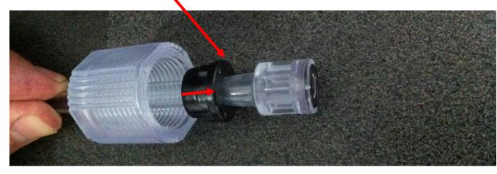
Now we attach the suction line fittings back into the pump head.
