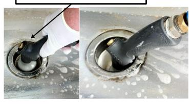
• Turn the wash gun back on, select the disinfect option (option 9) on the Key Pad and wash the under-floor area, return tilt floor to the down position. While still on disinfect, wash down the tub area of the dog wash. Turn gun off, remove wash down key and select the stop option on the Key Pad.
