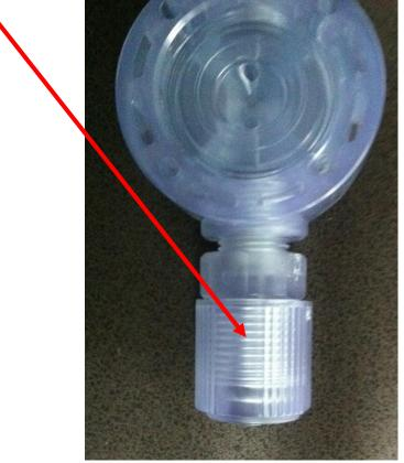
The first pieces we see when the fitting nut is removed are the: Hose adaptor and Hose stopper.
