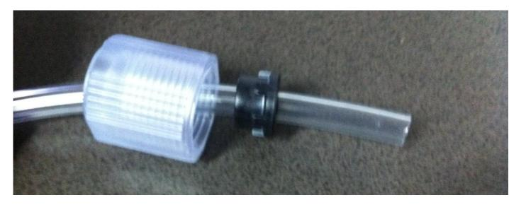
Push the hose onto the hose adaptor so that it is flush, this is vital to ensure a good seal.
