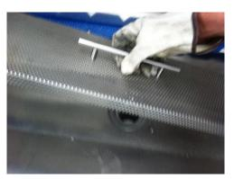
Warning the stainless-steel filter can have sharp edges, "rigger" gloves need to be worn to protect against injury. If required, you can wear rubber gloves underneath the "rigger" gloves.
