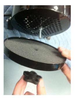
These pictures show the position of the filter requiring cleaning and how to access it. Ensure power disconnected and that the dryer is cool prior to commencing task. The internal dryer clamps should be checked every 3 months to ensure that the dryer pipes do not become loose. If either connection is found to be loose use a screw driver to tighten the screws that hold it in place.
