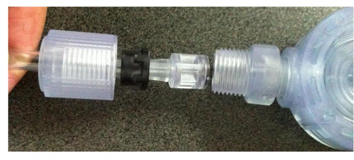
As we tighten the fitting nut the hose stopper will close up on the hose adaptor and the task is complete.
