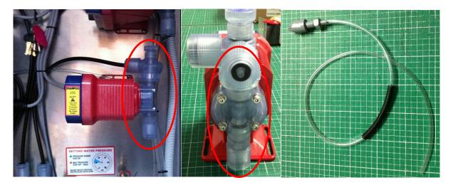
Prior to attaching the suction line to the pump, attach it to the soap management system.
